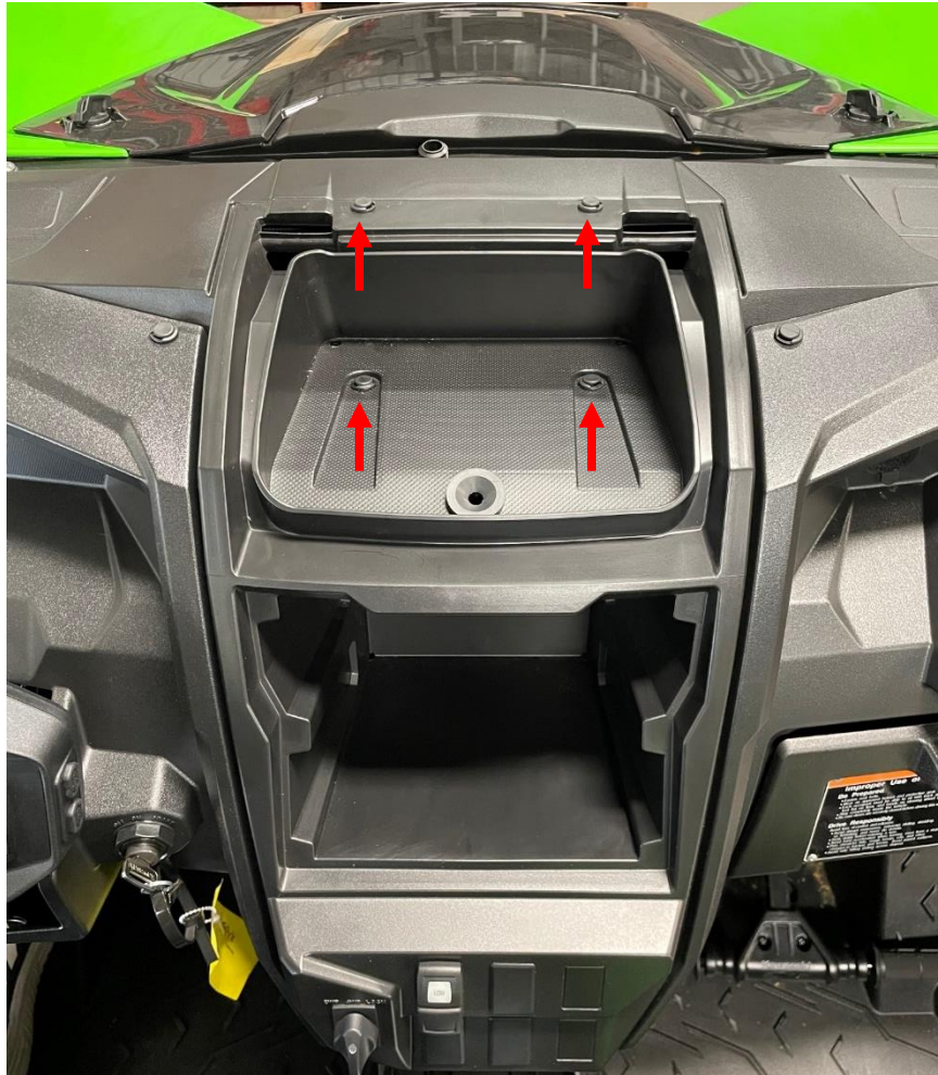
Figure 6: Remove the plastic rivets in the center dash.
