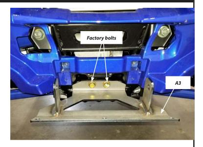
6. Attach the upper bumper support (A1) using the M12 hardware (B3 & B4). NOTE: Slide the bolt up through the frame and attach the nut topside. Do not tighten completely to allow for adjustment.
