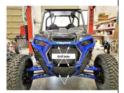
4. If nut plate should fall in step one, remove the two torx head screws shown. Pull outward on plastic and retrieve the nut plate with a magnet.
