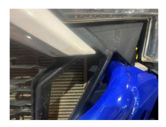
STEP 4: Using the bolts removed in step 2, start the lower bolts but do not tighten.
