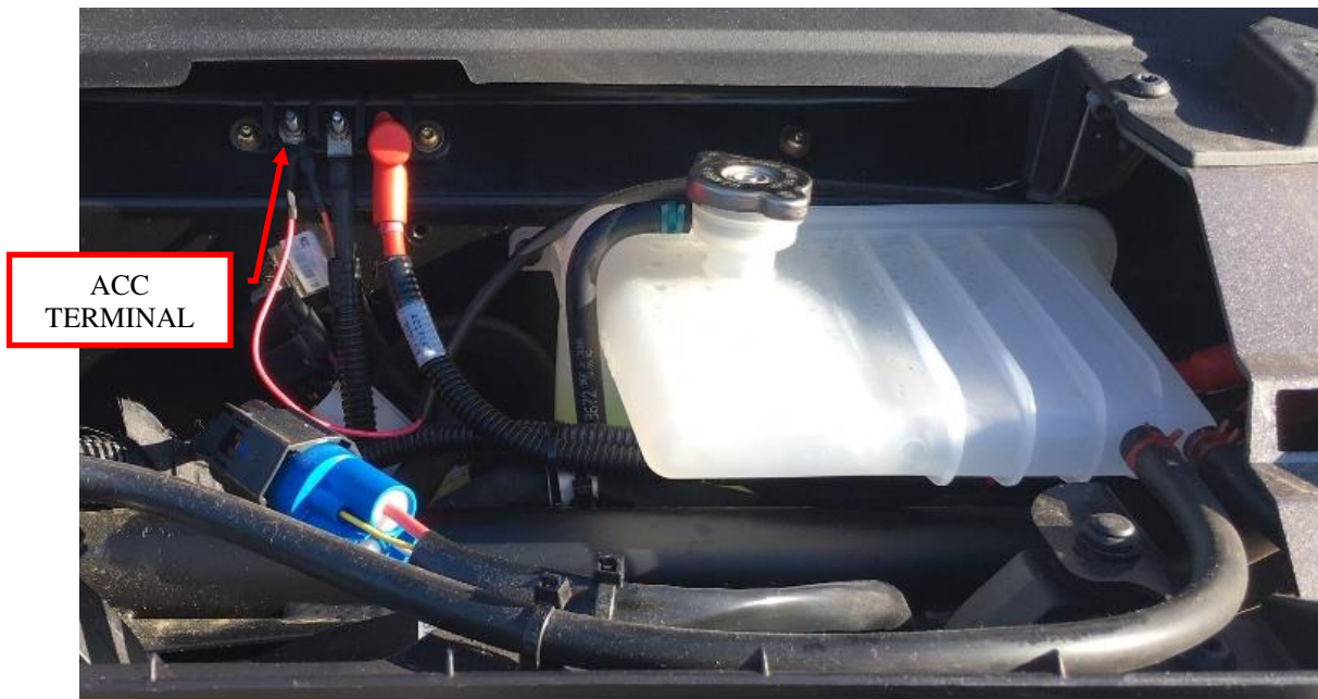
Figure 11: Connect to the ACC terminal.
