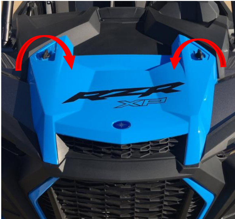
Figure 9: Remove the radiator hood access panel.
