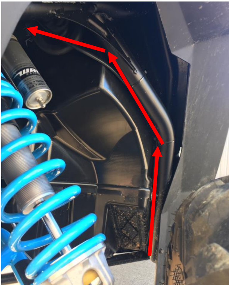
Figure 10: Wire routing in front fender.
