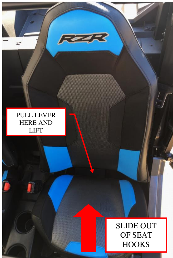
Figure 6: Remove the rear driver's side seat.
