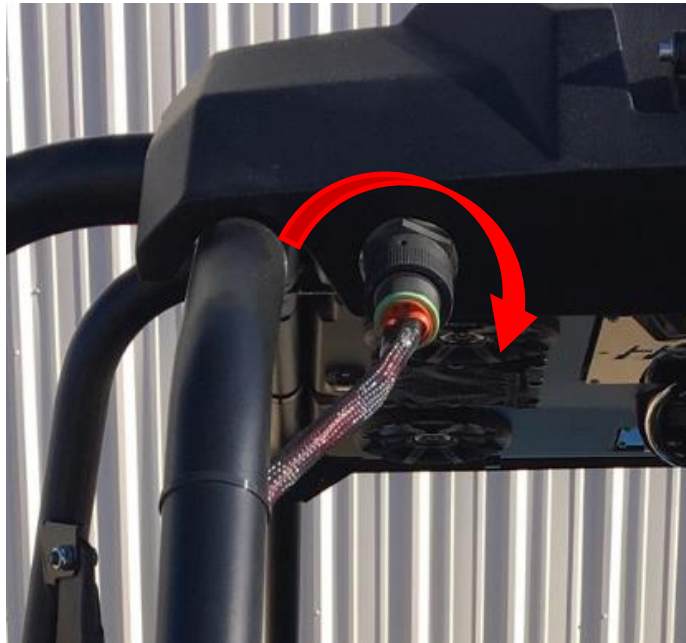
Figure 12: Align connector terminals and rotate 1/4 turn.
