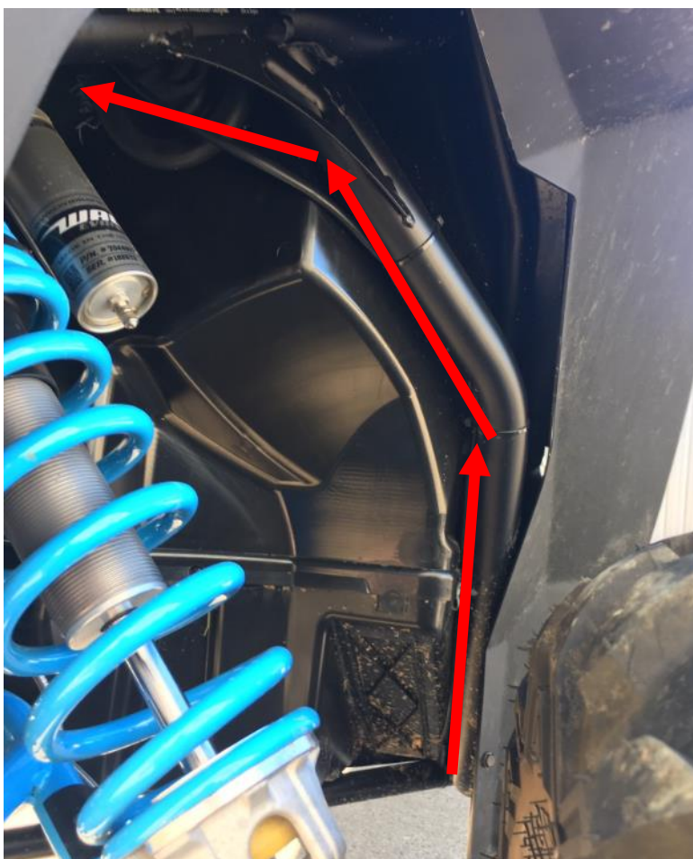
Figure 10: Wire routing in front fender.
