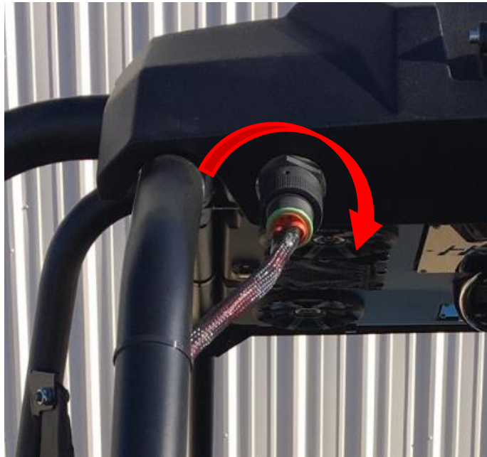
Figure 12: Align connector terminals and rotate 1/4 turn.
