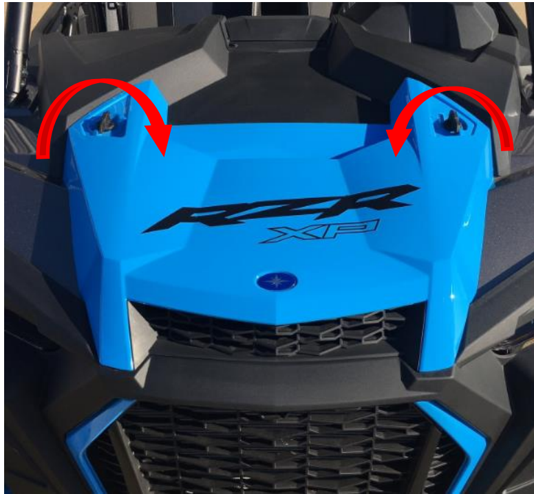
Figure 9: Remove the radiator hood access panel.
