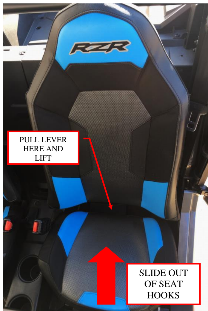
Figure 6: Remove the rear driver's side seat.
