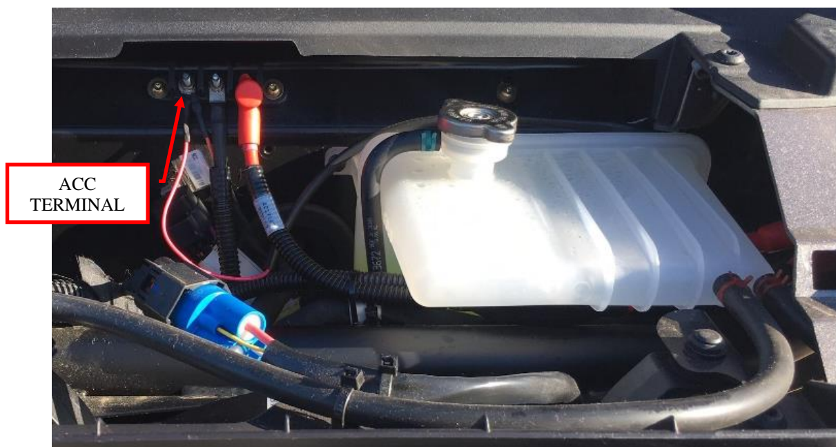
Figure 11: Connect to the ACC terminal.
