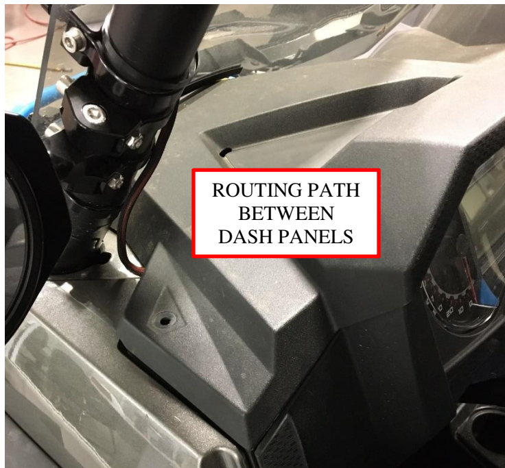
Figure 13: Harness routing between dash panels.
