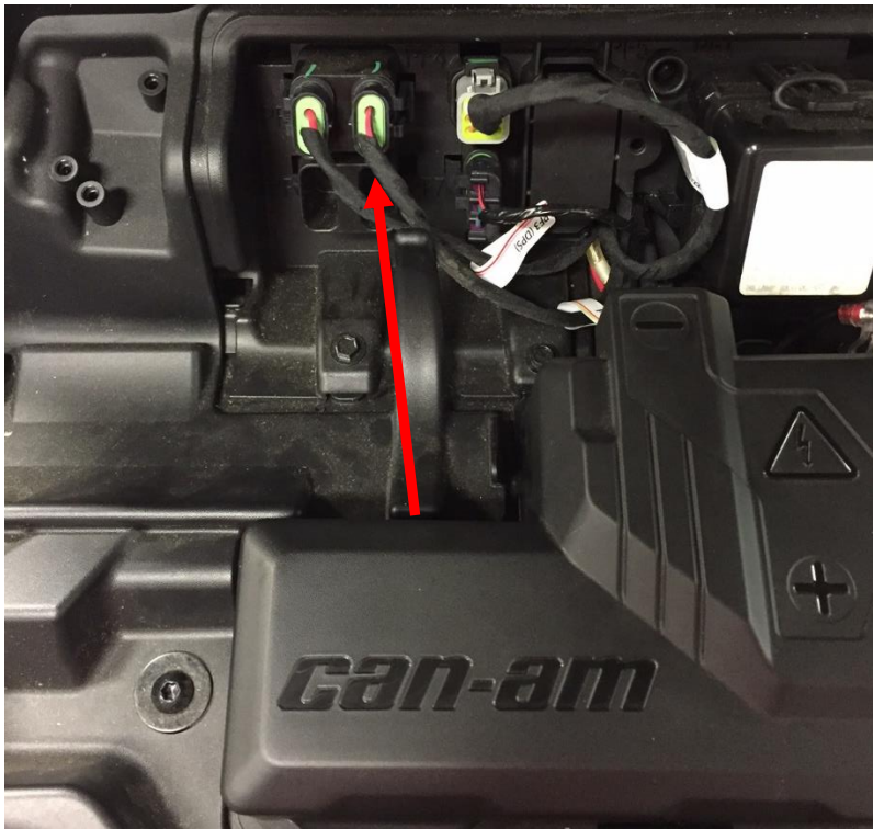
Figure 14: Accessory port connection.
