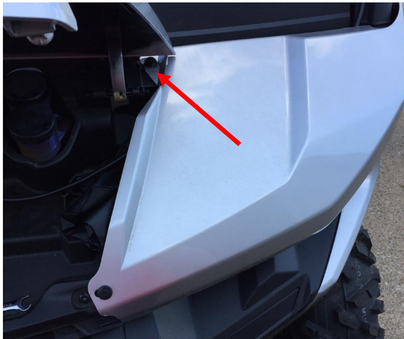
Figure 13: Remove the plastic rivet to run the chassis harness under the panel.
