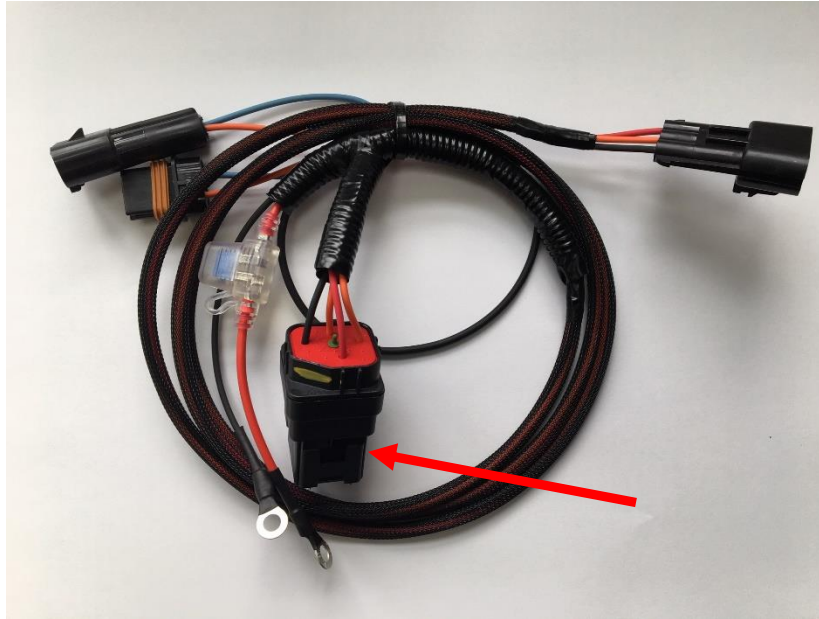
Figure 2: Chassis harness ignition relay
