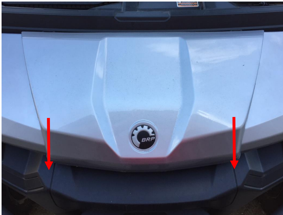
Figure 12: Lift the radiator hood access panel.
