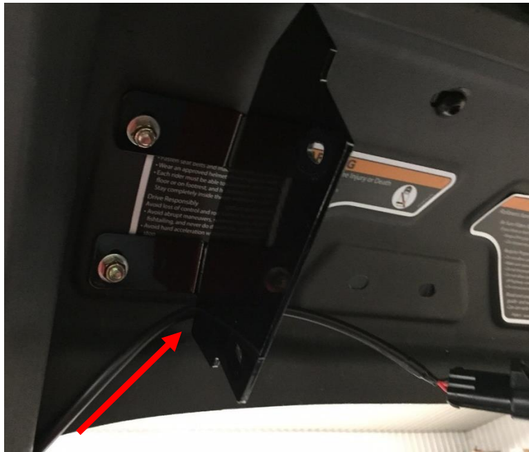
Figure 5: Placement of the chassis harness connector before mounting the unit.
