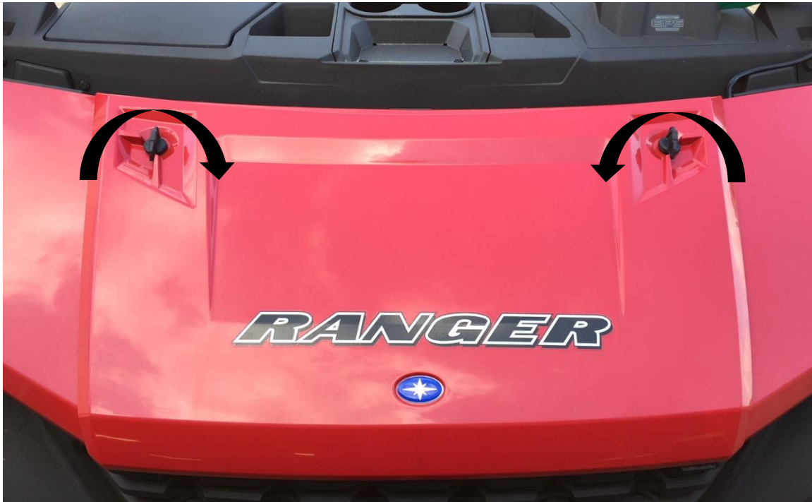
Figure 14: Remove the radiator hood access panel.
