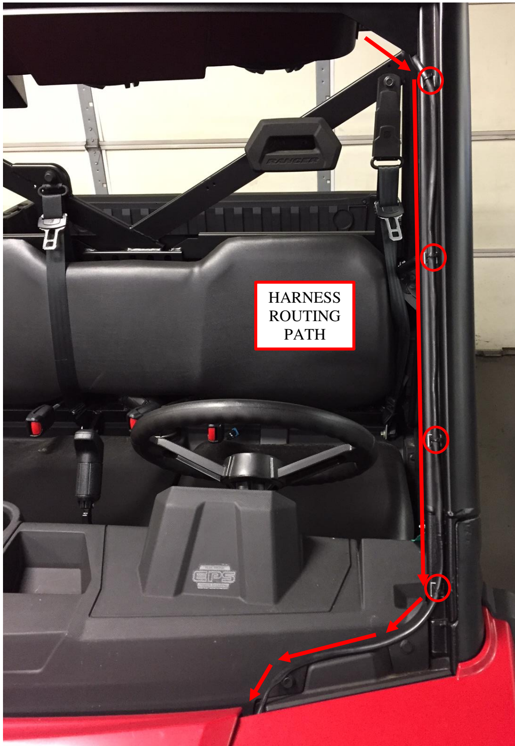
Figure 13: Route the chassis harness down the driver's front pillar.
