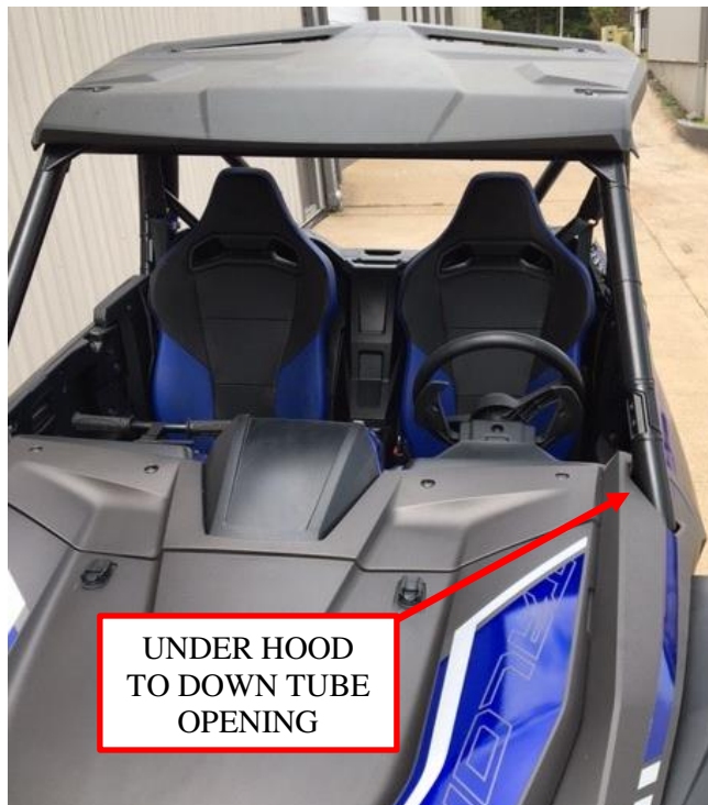
Figure 10: Chassis harness routing under hood to opening.
