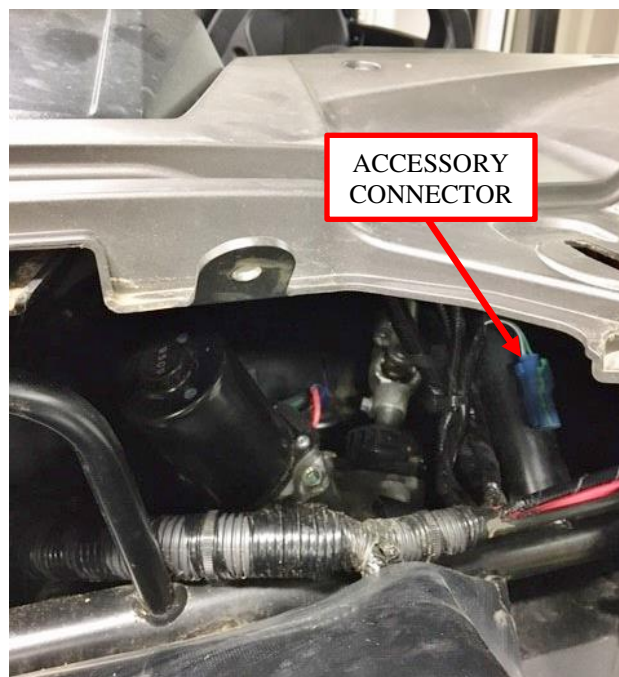
Figure 8: Factory accessory connector location.
