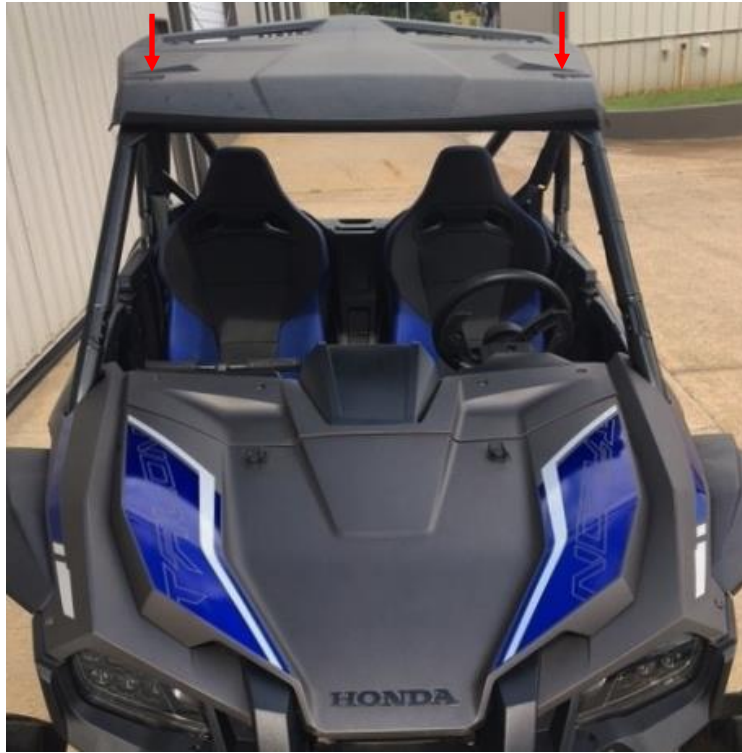
Figure 2: Remove front bolts attaching the roof to the frame.
