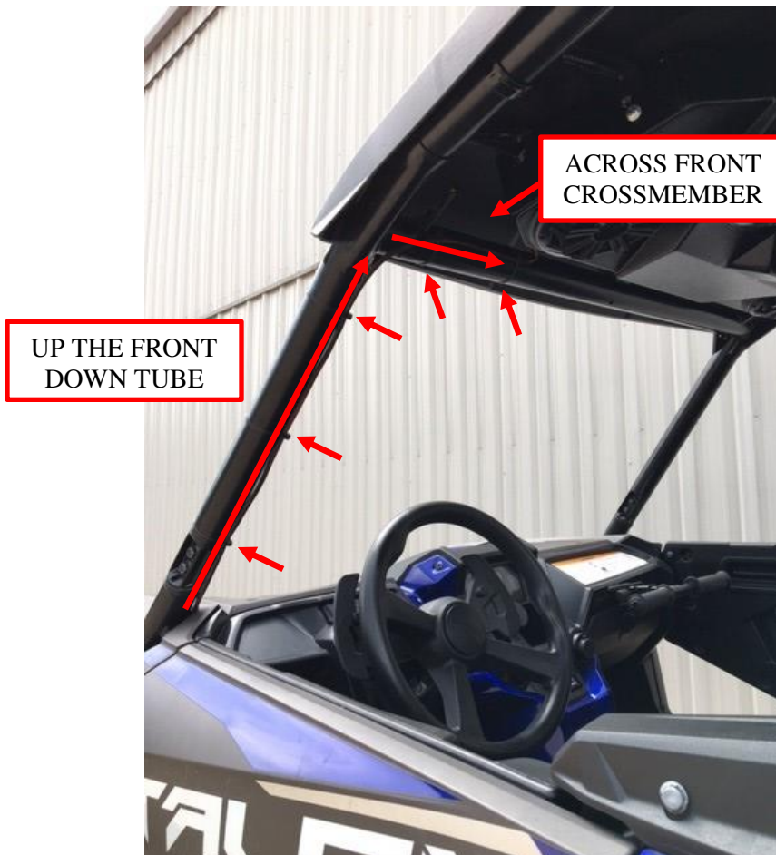
Figure 11: Chassis harness routing up driver's front down tube.
