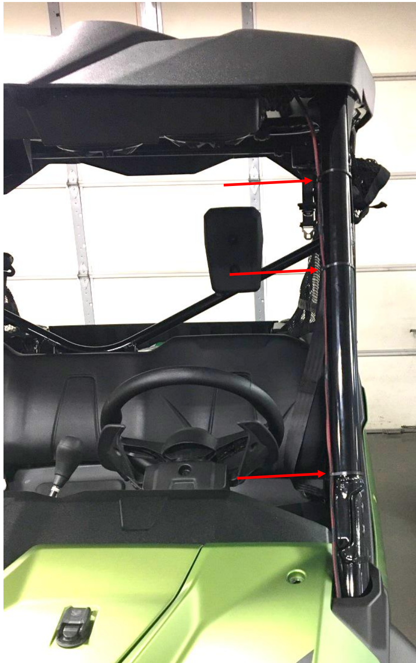
Figure 11: Route the chassis harness down the driver's front pillar.
