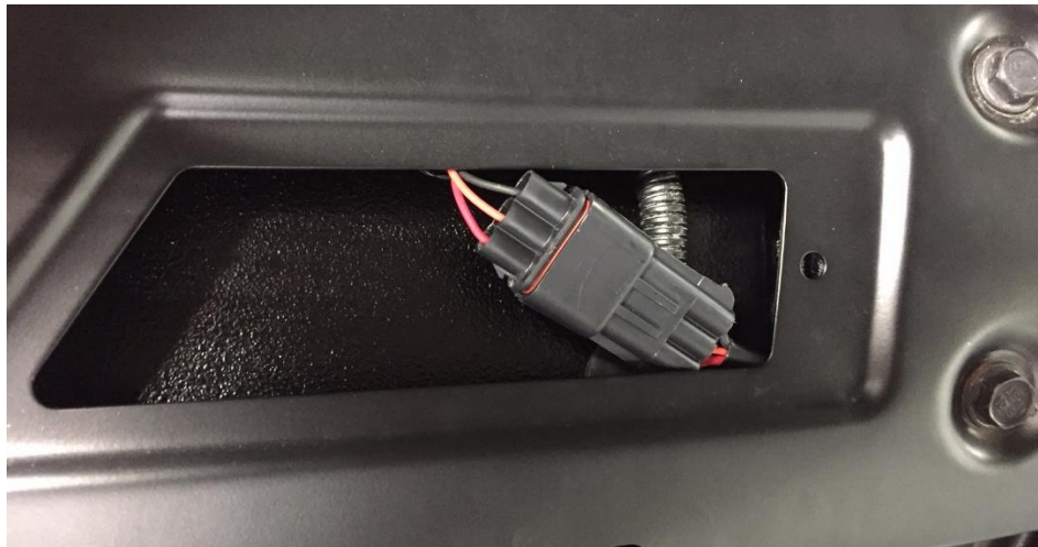
Figure 8: Connect the chassis harness to the sound system.
