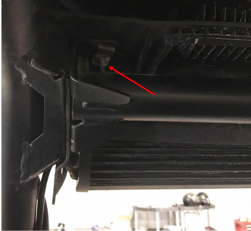
Figure 2: Remove screw to access cross member bolt.
