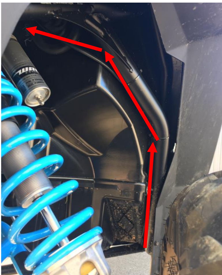
Figure 10: Wire routing in front fender.
