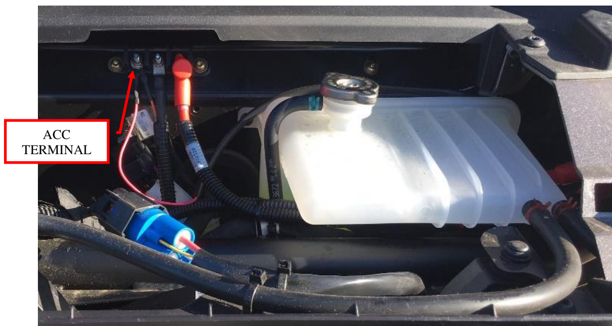
Figure 11: Connect to the ACC terminal.
