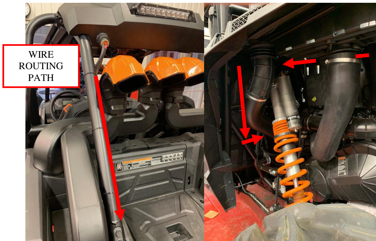
Figure 7: Route the battery cable wiring.
