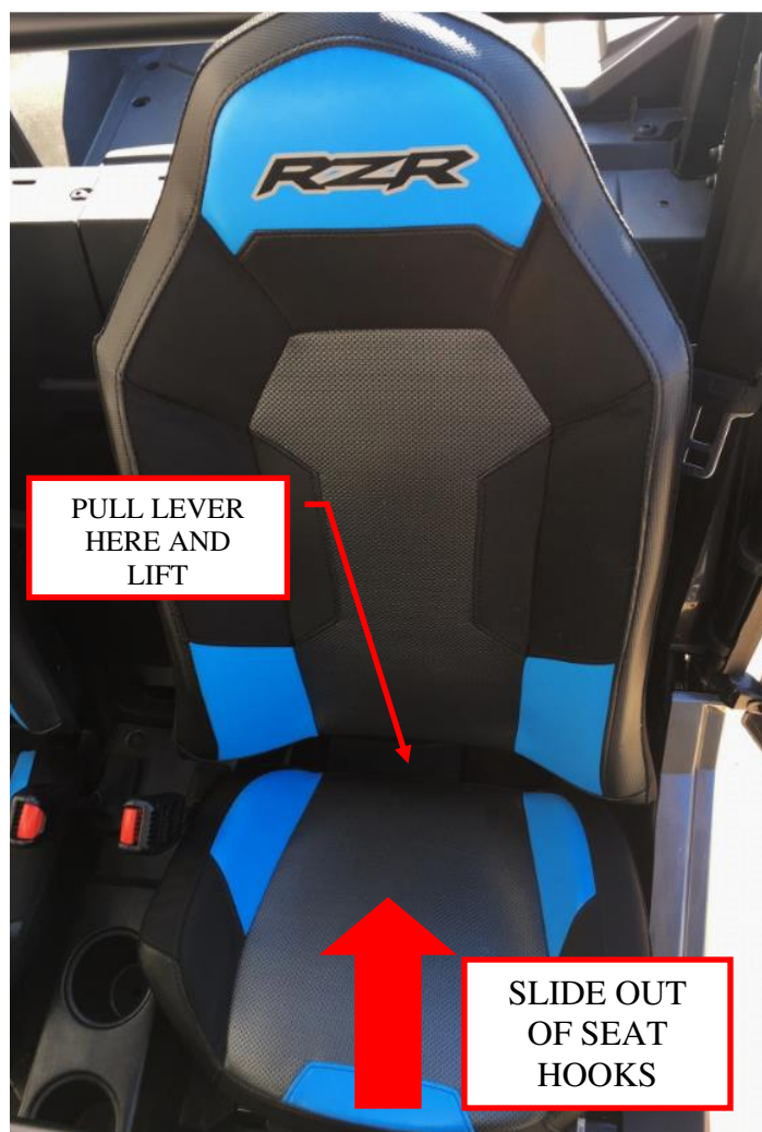
Figure 6: Remove the rear driver's side seat.
