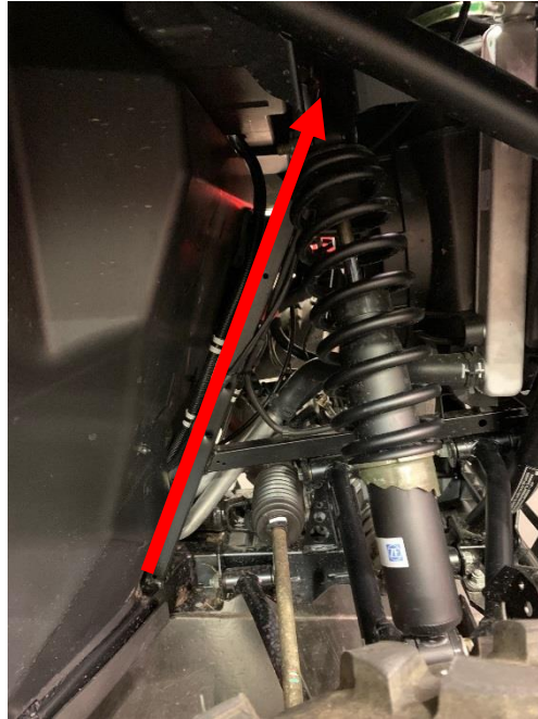
Figure 11: Wire routing in front fender.
