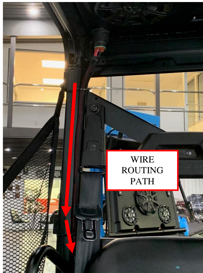
Figure 7: Route the battery cable wiring.
