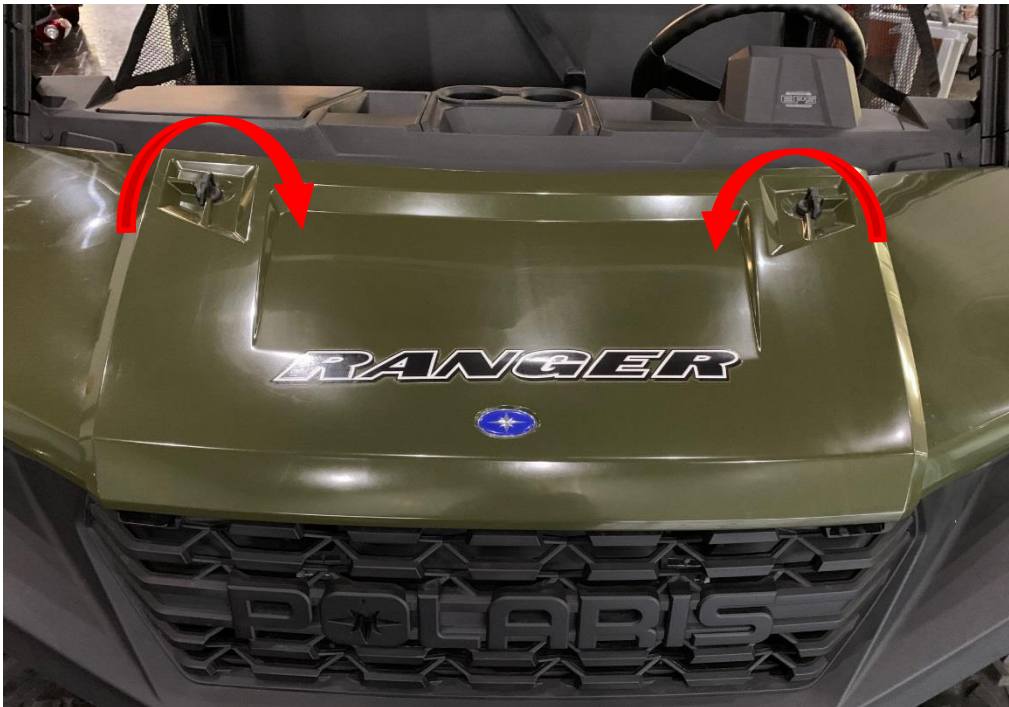
Figure 9: Remove the radiator hood access panel.
