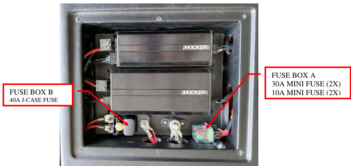
Figure 1: Fuse location.
