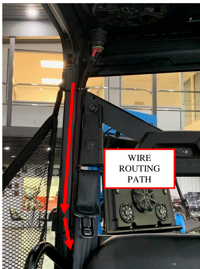
Figure 10: Route the battery cable wiring.
