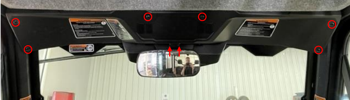
Figure 3: Remove the front roof liner.
