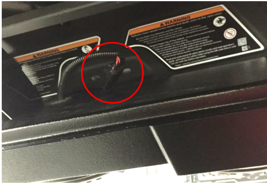
Figure 17: Harness connection on top of unit before mounting.
