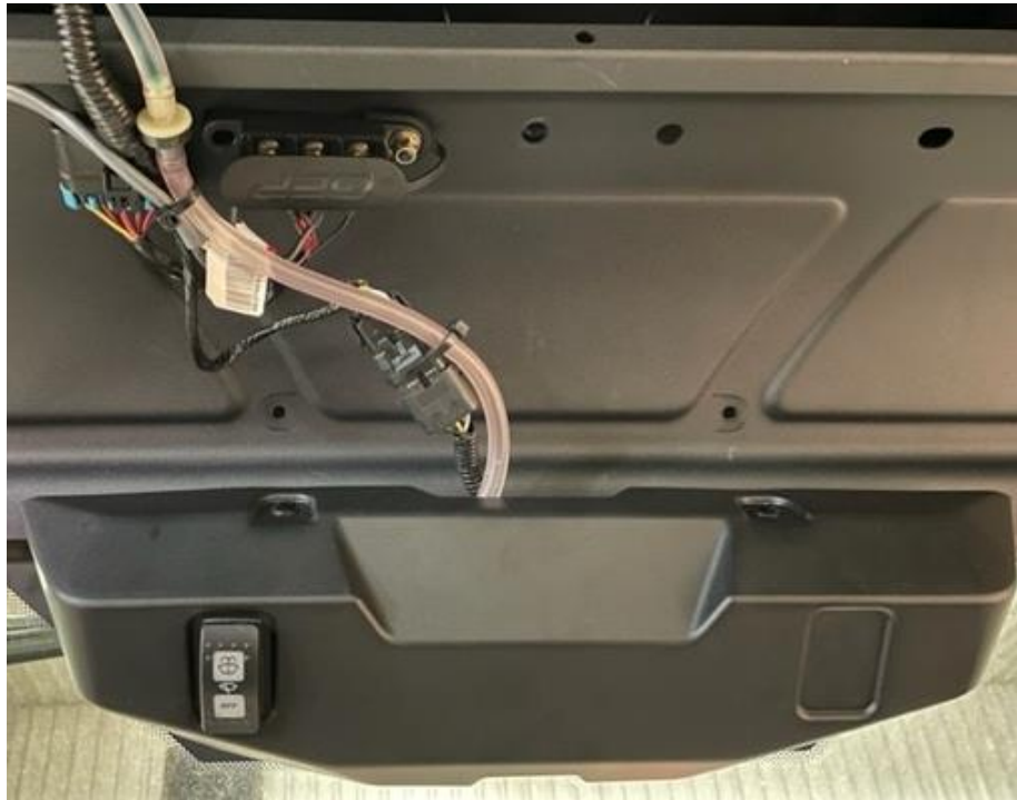
Figure 13: Harness items mounted to visor.
