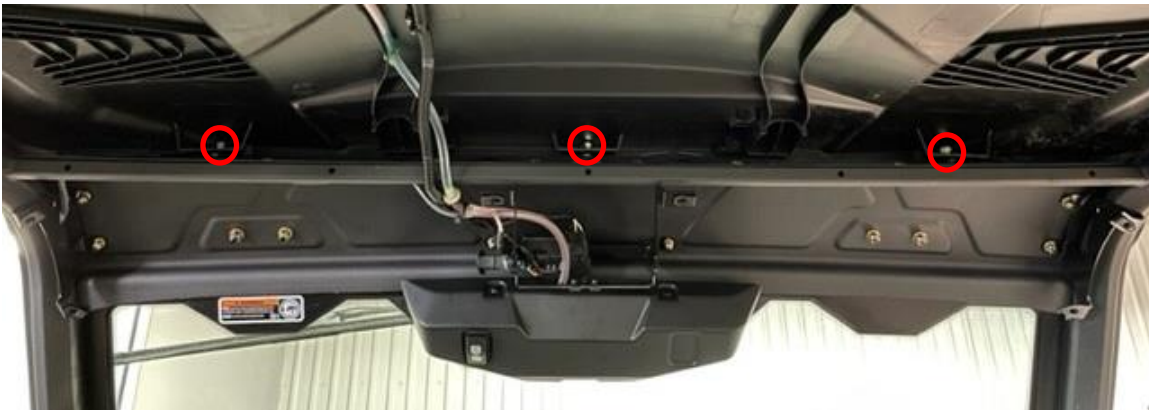
Figure 8: Remove 3 bolts to loosen the roof.
