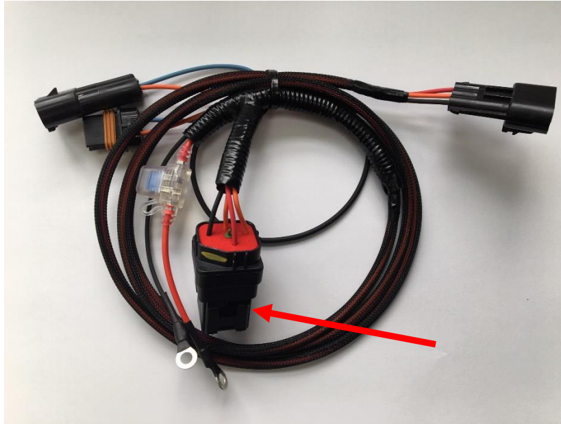
Figure 2: Chassis harness ignition relay
