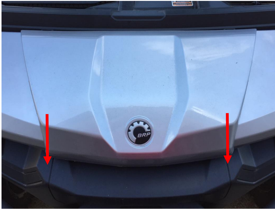
Figure 25: Lift the radiator hood access panel.
