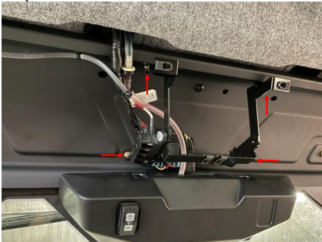
Figure 10: Remove the center roof liner bracket.
