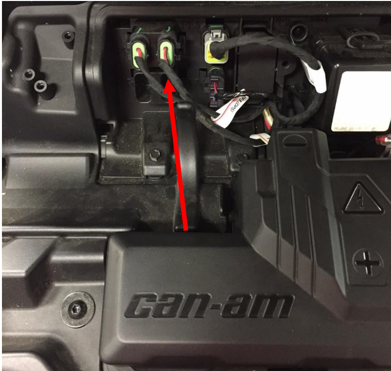
Figure 27: Accessory port connection.
