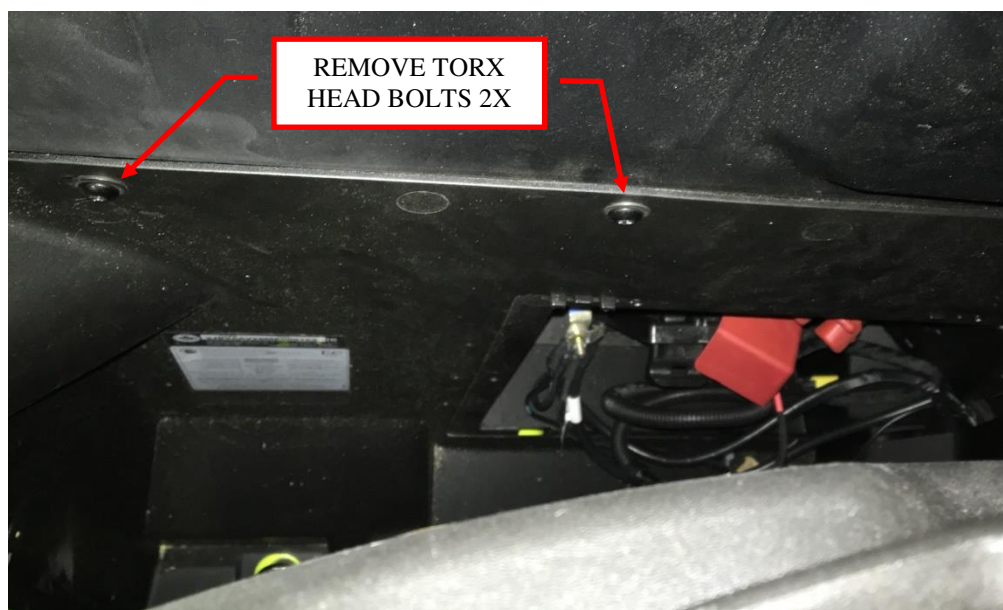
Figure 8: Remove torx bolts in rear firewall.
