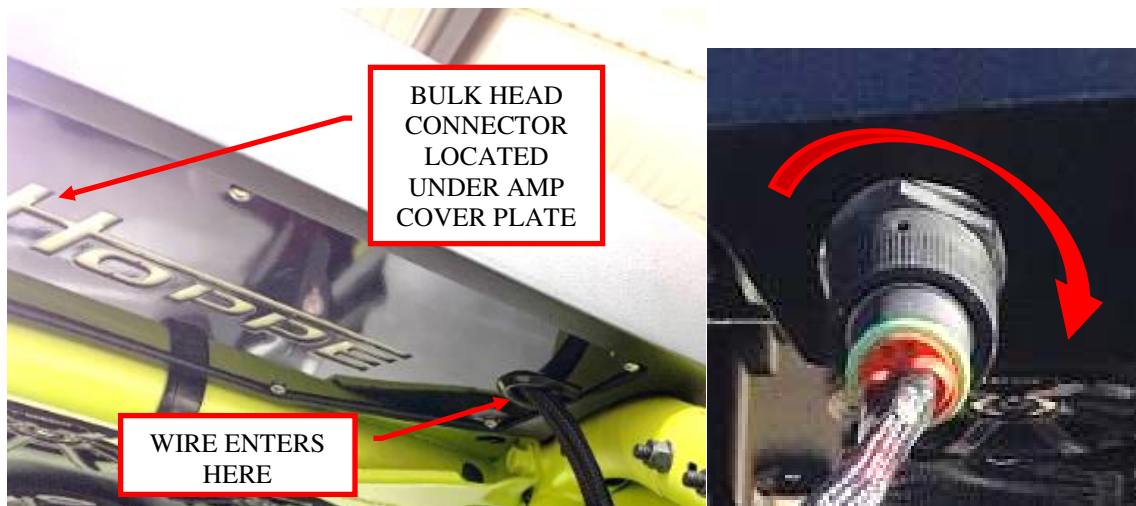
Figure 13: Align connector terminals and rotate 1/4 turn.
