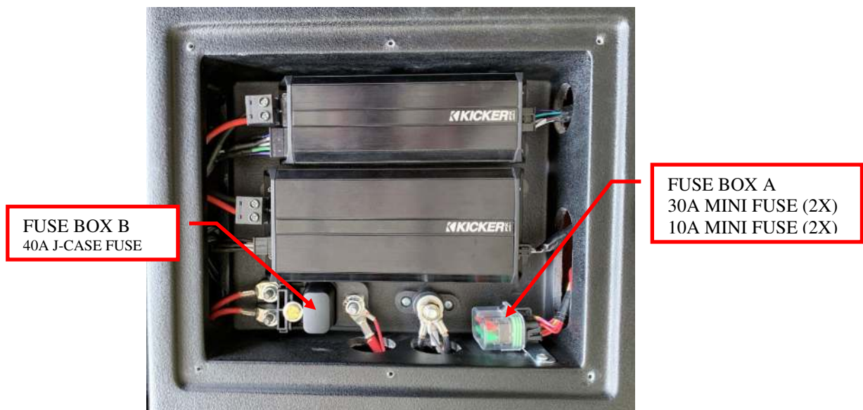
Figure 1: Fuse location.
