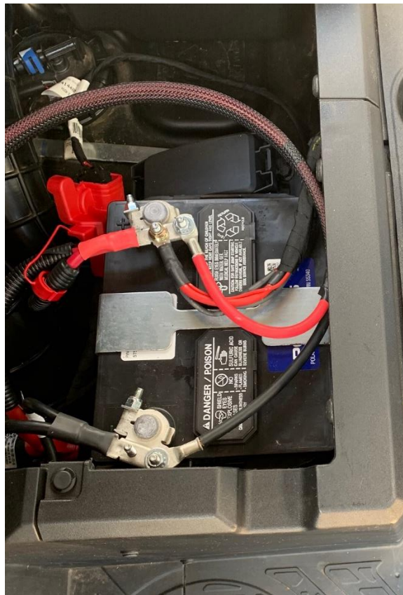
Figure 9: Fold seat forward and remove tray for battery access.
