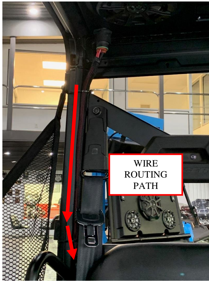
Figure 10: Route the battery cable wiring.
