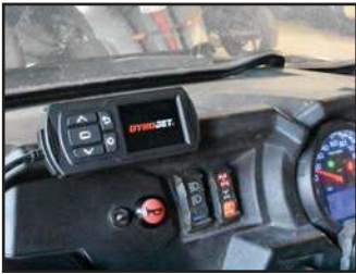
INSTALL POWER VISION
