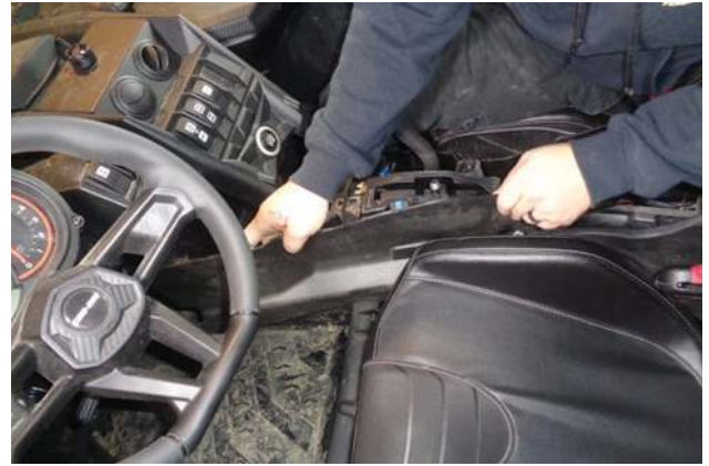
15. Remove both front side panels.
