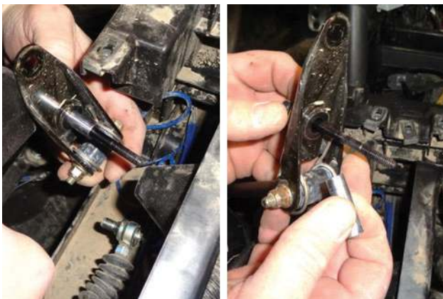
20. Remove pivot bushing.
