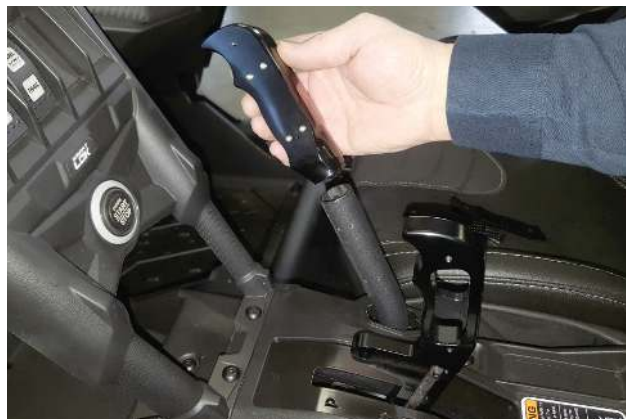
45. Install magnum grip grab handle (13) then cover plates and screws.
