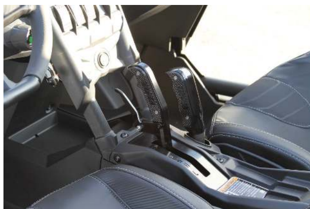
46. Install lock nut, shoulder bolt, spring washer and shift lever (removed step 40) onto shifter stick. Then install shifter both plate cover and screws (x4) (removed step 39).
