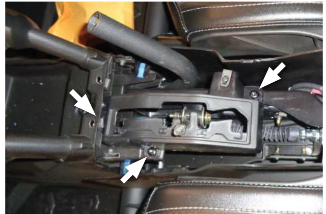
16. Move shifter into "Neutral". Remove and retain screws (x3) then shifter gate.
