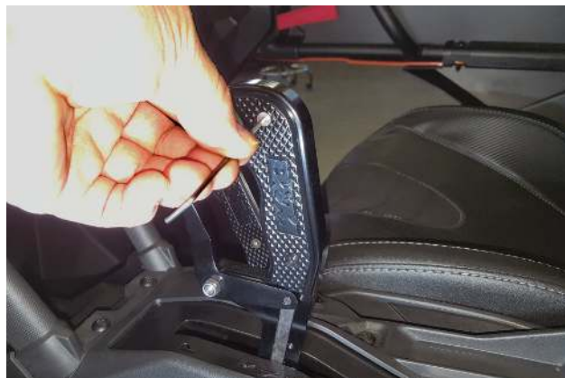
46. Install lock nut, shoulder bolt, spring washer and shift lever (removed step 40) onto shifter stick. Then install shifter both plate cover and screws (x4) (removed step 39).
