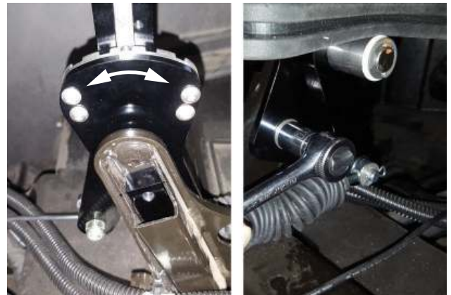
17. Center shifter in gear as shown then finish tightening gate mount to backer bar.
