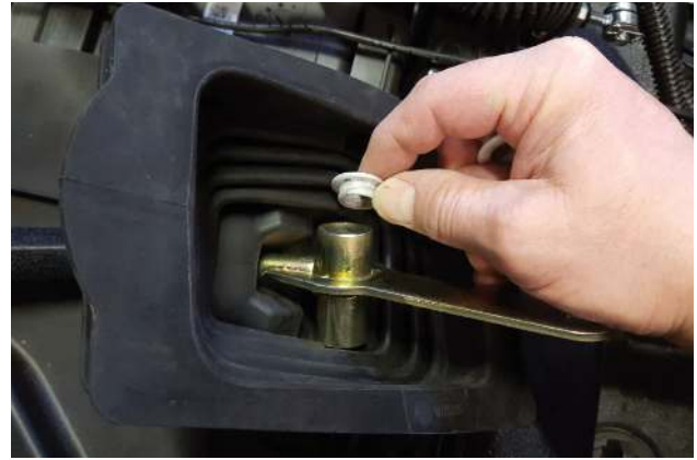
9. Remove and retain bushings (x2) from shift lever.
