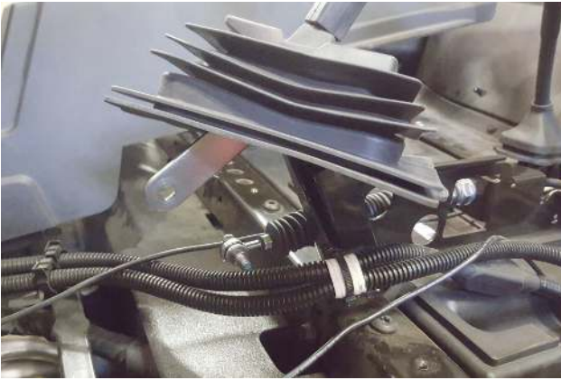
6. Remove and retain shift cable lock nut then disconnect cable from shift lever.
