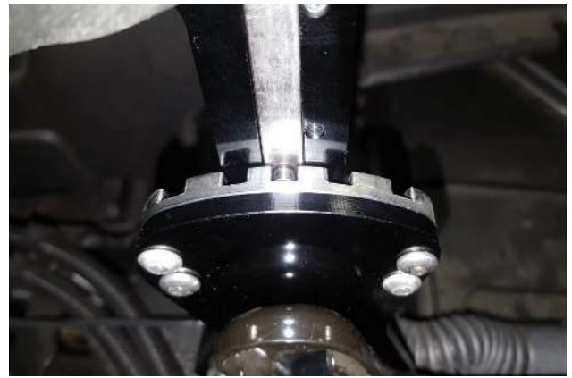
15. Now set pin selector into gear shown above.
