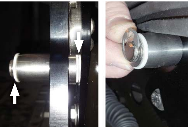
14. Place stick onto pivot shaft. Install as many shims (2) as necessary onto either side of pivot sleeve until shifter operation is smooth (no drag against gate plate) without too much play. Then secure it in place using e-clip (removed step 7).
