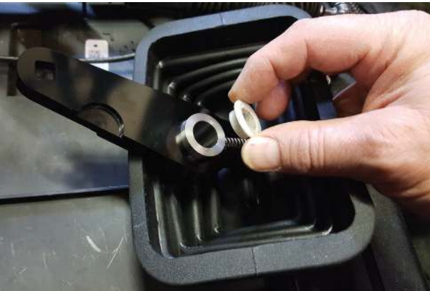
13. Assemble bushings (x2) (removed step 9) into both ends of pivot sleeve on stick (1) .
