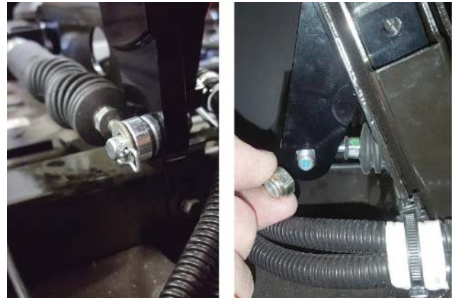
16. Re-connect shift cable then secure it using shift cable lock nut (removed step 6).
