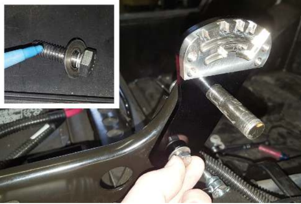
12. Apply loctite to screw (7) then insert it through flat washer (8) , gate mount and backer bar to secure parts together. Hand tighten screw loosely.
