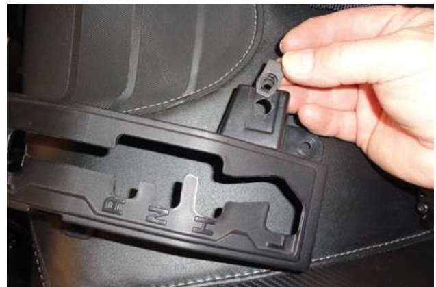
17. Remove nut plate from passenger side of shifter gate. Retain it for later use.
