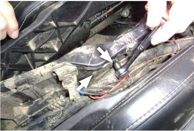
25. Remove screws (x2) securing right side of cable support.
