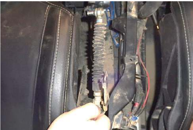
26. Lift cable support out of frame.
