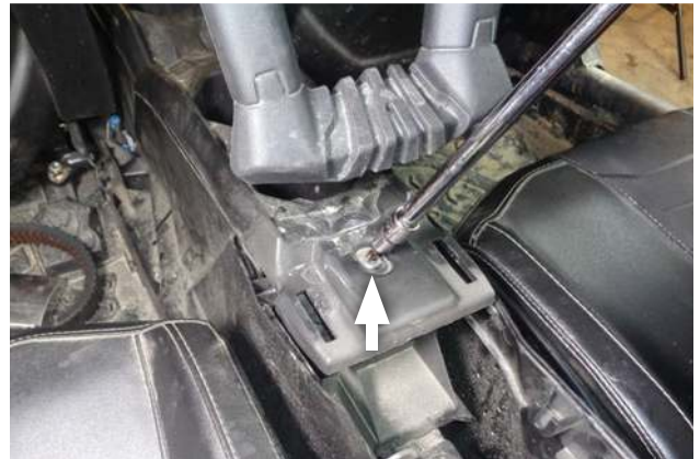
10. Remove screw at rear of middle console cover.
