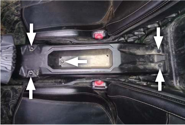
6. Slide frong seats fully forward. At rear of console cover, remove screws (x3) and push rivets (x2).
