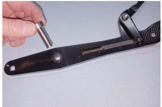
29. Install plastic sleeves (x2) (removed step 21) then spacer (9) onto shifter stick (1).
