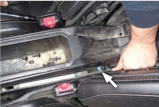
7. Unsnap clip securing rear of each rear side panel to rear console cover.
