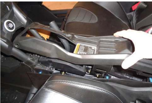
14. Unsnap clips (x3) on front side panels, then remove front console cover.
