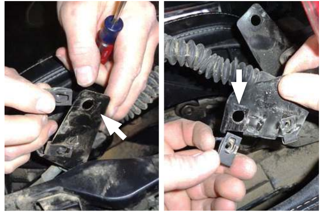
27. Remove nut plates (x2) at front of shifter support.
