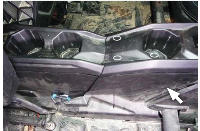
9. Gain access to screws (x3) securing front of middle console cover as follows (Steps 10-12).
