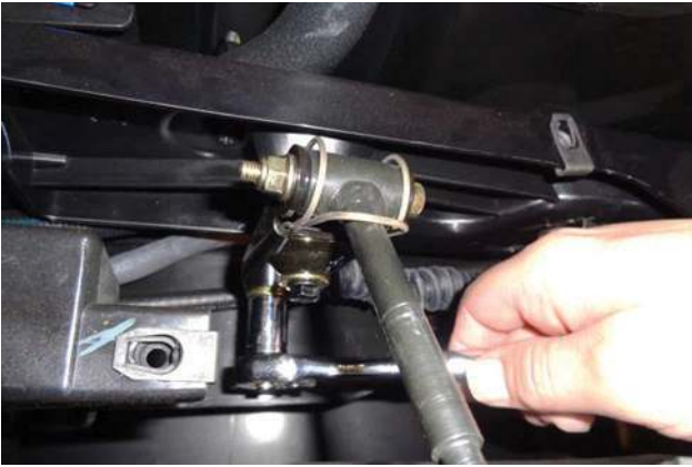
18. Remove nut and washer connecting shift lever to cable. Retain nut for later use.
