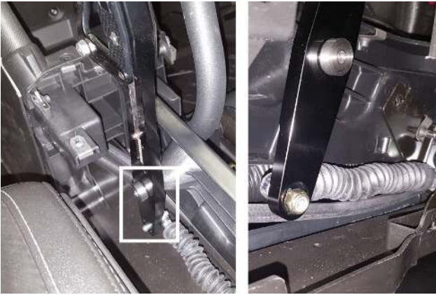
30. Install shifter stick by inserting spacer through pivot bore then secure shifter cable by tightening nut (removed step 19).
