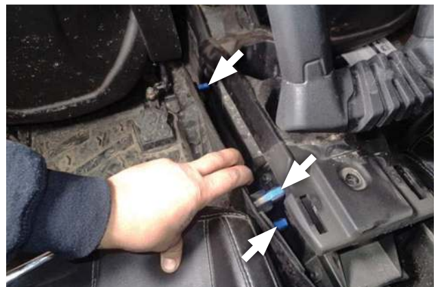
11. Unsnap clips (x3) and remove both middle side panels.
