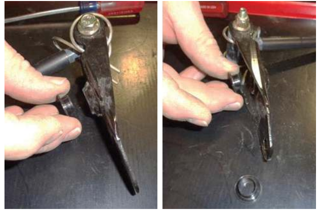
21. Remove and retain plastic sleeves (x2) from shifter.
