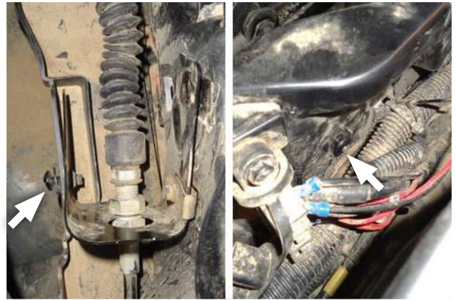
28. Reinstall cable support into frame. Hand-start (do not tighten) only rear screws (x2).
