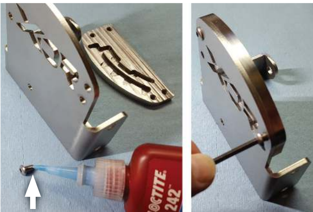
31. Apply loctite to screws (x4) and use them to fasten gate mount (2) to gate plate (4).
