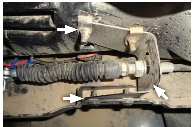
23. Remove nut plates (x2) at front of shift cable support as follows (Steps 23-26).
