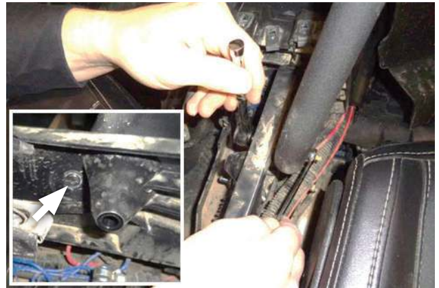
22. Remove screw, nut and washer securing grab handle tube to frame. Retain fasteners for later use.
