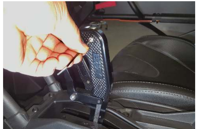
46. Install lock nut, shoulder bolt, spring washer and shift lever (removed step 40) onto shifter stick. Then install shifter both plate cover and screws (x4) (removed step 39).
