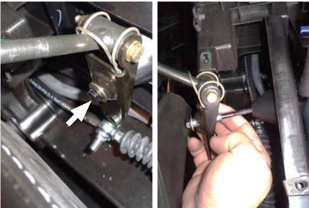
19. Remove shift lever pivot screw, nut and washers, then shift lever. Retain screw and washer for later use.
