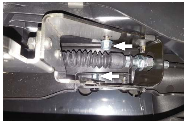
35. Secure gate mount bracket to cable support using screws (removed steps 23-25). Fasten components loosely using nuts (x2) (10).
