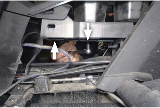
12. Remove screws (x3) under front cup holder in middle console cover.
