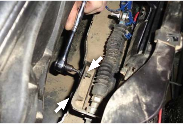
24. Remove screws (x2) securing left side of cable support.
