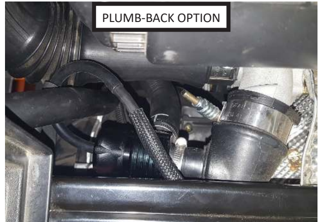
15. Plumb-back option: for quieter operation, install blow-off valve as shown leaving out breather filter.
