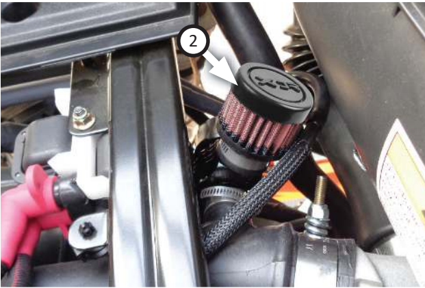
13. Install breather filter (2) onto blow off valve, then tighten it just enough to allow for later adjustment.
