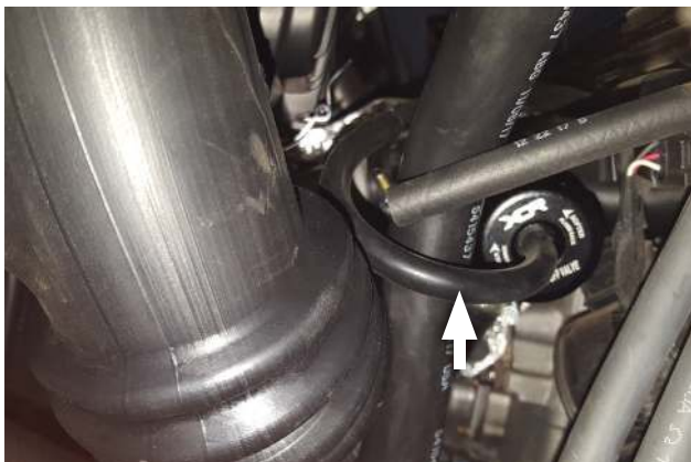
12. Route vacuum hose down around vent tube then connect it to blow off valve.
