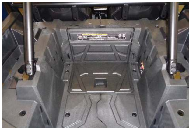
16. Replace cover on air box compartment.
