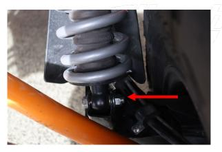
Loosen and remove the hardware that secures the coilover to the control arm. Note: Never work on or under a vehicle that is not supported by the proper safety equipment.
