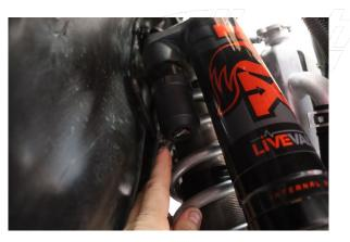
Plug in the electrical connector at the top of the coilover.
