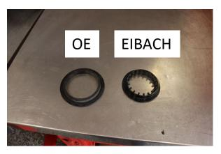
Remove the OE Spring adapter and replace with the provided one. Then reinstall the crossover ring and slider sleeve with the clips.
