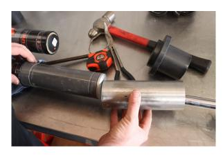
Remove the slider sleeve and crossover rings.
