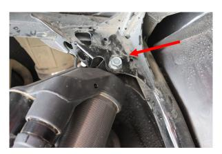
Loosen and remove the hardware that secures the coilover to the upper mount.
