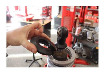
Step 5. Compress the coilover, then remove the OE spring retainer. **Note: The bump stop will need to be pried down, out of the way of the spring retainer.**
