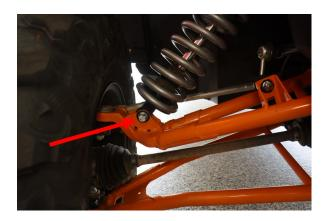
Loosen and remove lower front shock hardware.
