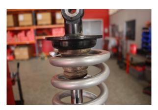
Compress the spring assembly and re-install the spring retainer.
