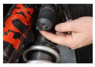
Remove electrical connector from the top of the coilover.
