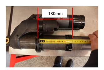
Install the cross-over rings and set them at **130mm** measuring from the spring flange to the bottom of the crossover ring.
