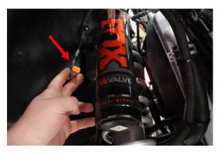
Disconnect the electrical connector at the top of the coilover.
