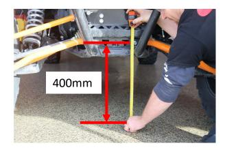
Measure from the ground to the center of the lower radius arm bolt. The recommended preload measurement will get the vehicle close to the recommended ride height with extra weight added, but each vehicle may vary some. We recommend setting the ride height at **400mm** measuring from a flat surface to the center of the lower control arm bolt. Rear shock length is approximately **918mm** eye to eye at ride height.
