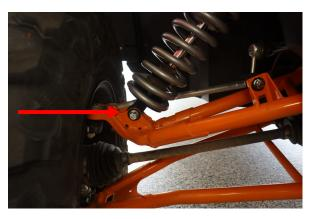
Secure the coilover to the control arm with the OE hardware.
