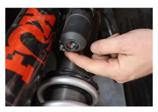
Reinstall the connectors at the top of the shock for the Live Valve and complete on the opposite side.
