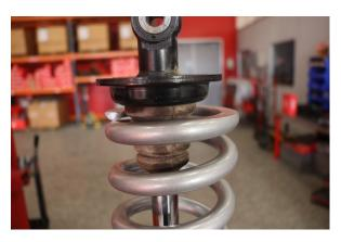
Step 5. Compress the coilover, then remove the spring retainer. **Note: The bump stop will need to be pried down, out of the way of the spring retainer.**
