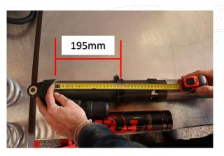
Set the preload collar to 195mm measuring from the base of the reservoir housing to the spring perch.
