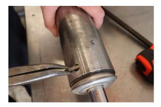
Remove the inner flat retaining wire through the access hole of the slider sleeve. Be sure not to distort of bend this wire as it will go back when finished.
