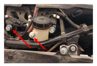
Loosen and remove the hardware that secures the coilover to the upper mount.
