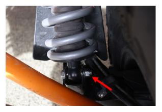
Install the bolt connecting the shock to the lower control arm.
