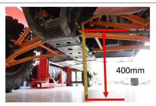
Lower vehicle back to ground and measure from the ground to the center of the lower control arm bolt. The recommended preload measurement will get the vehicle close to the recommended ride height with weight added to the vehicle, but each vehicle may vary some. We recommend setting the ride height at 400mm measuring from a flat surface to the center of the lower control arm bolt.. Front shock length is approximately 735mm eye to eye at ride height
