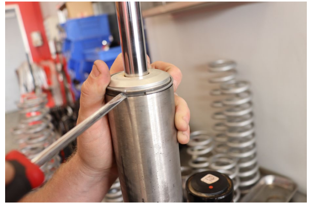
Remove the clip at the end of the shock body securing the slider sleeve.
