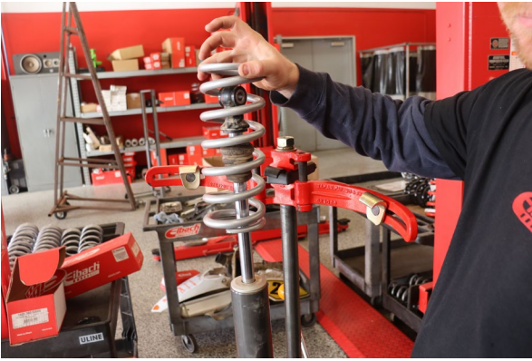
Install the Eibach secondary spring.
