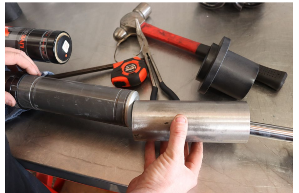
Remove the slider sleeve and crossover rings.
