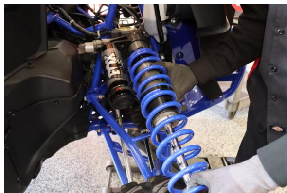
Step 6. Remove the coilover.
