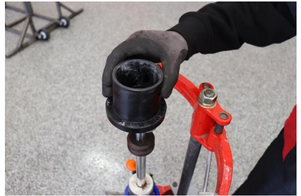
Step10. Remove OE slider.
