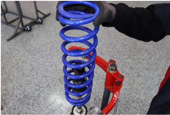
Step 9. Remove OE main spring.
