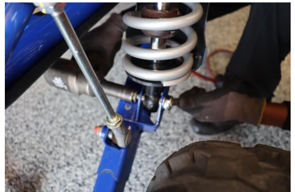
Step 18. Re-install the coilover.
