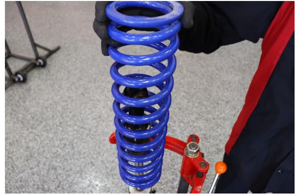
Step 8. Remove OE main spring.
