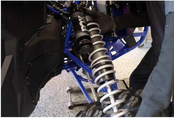
Step 19. Re-install coilover
