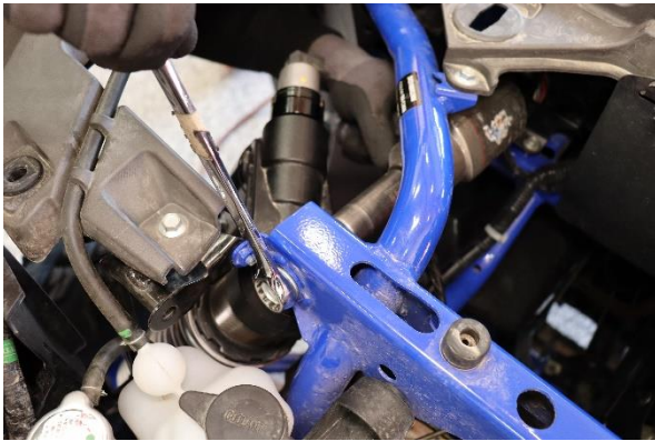
Step 21. Secure the coilover to the upper mount with the OE hardware.
