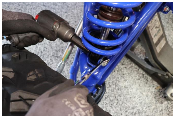
Step 2. Raise the front of the vehicle and support it with the proper safety equipment. Loosen and remove the hardware that secures the coilover to the control arm. Note: Never work on or under a vehicle that is not supported by the proper safety equipment.
