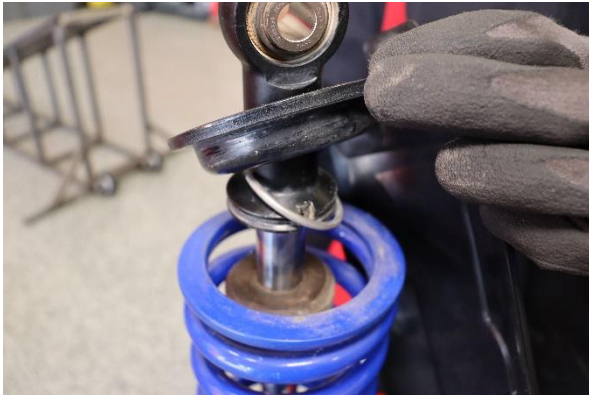
Step 7. Remove spring retainer.
