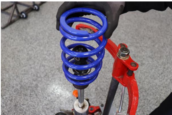
Step 11. Remove OE secondary spring.
