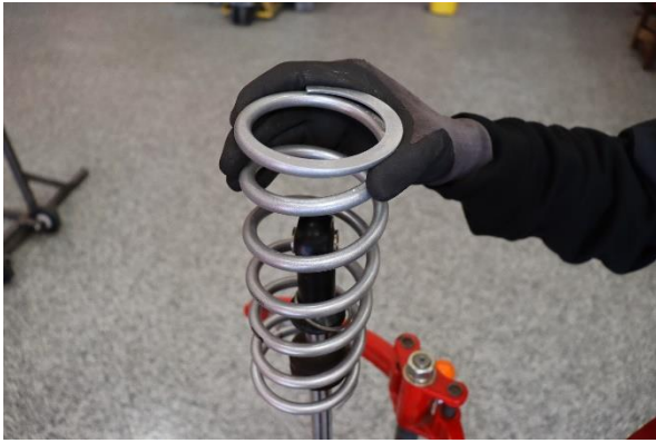
Step 13. Install the Eibach secondary spring.
