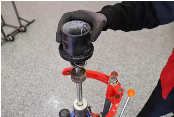
Step 9. Remove OE spring slider.
