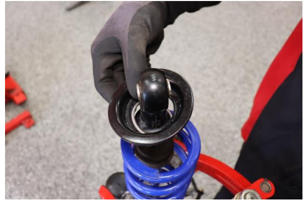
Step 8. Remove spring retainer.
