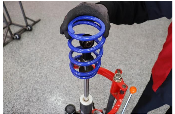
Step 10. Remove OE secondary spring.
