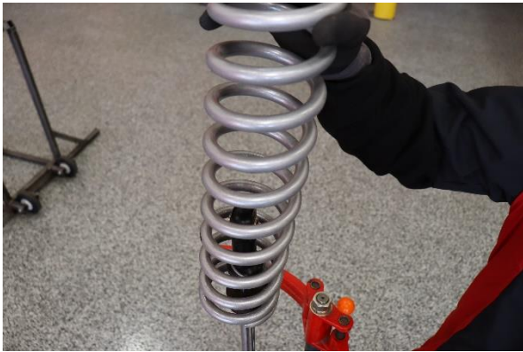
Step 15. Install the Eibach main spring.
