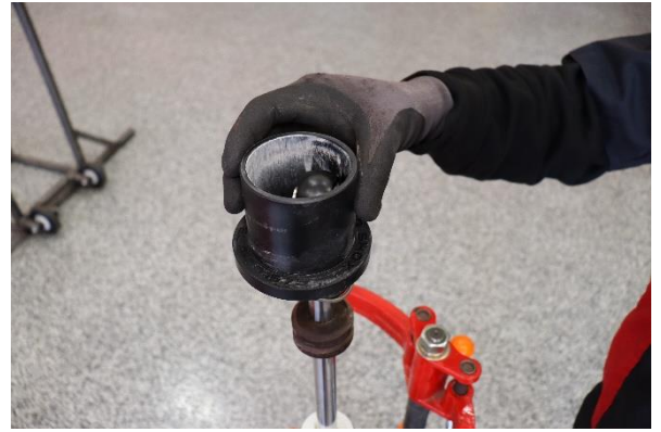
Step 14. Install the Eibach spring slider.
