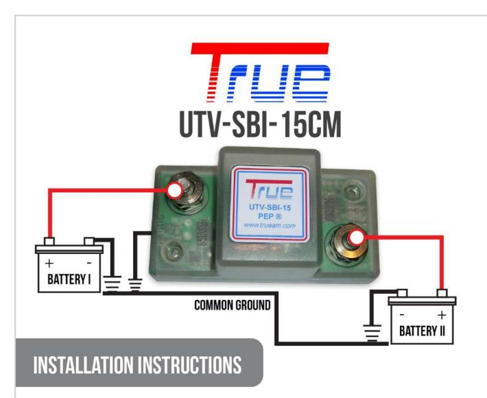
FYI: The SBI is designed ambidextrous so it cannot be installed backwards. Either stud can be connected to either battery's positive terminal.
