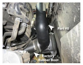
Beginning at the upper most factory boot on the CVT housing, install part #8 and orient as shown. This will be the center riser.
