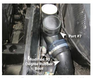
Next, install part #7 into the rubber boot with the small pipe on the larger end going into the boot.
