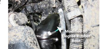
Beginning with the modified 90 degree rubber boot, insert the smaller cut end onto the air box tube.
