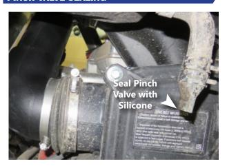
Apply silicone to the inside of the air box pinch valve to seal it.
