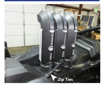
Install the Warrior Risers into the rubber boots and secure with hose clamps.
