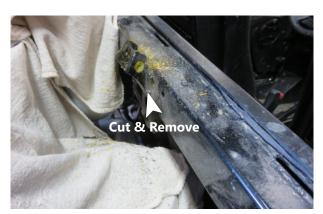
Locate this metal tab behind the seats, along the bed rail. Using a reciprocating saw, flush cut this tab and remove it to leave a smooth rail beneath.
