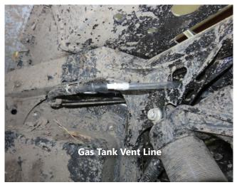
Using the clear tubing and barb couplings, extend the front differential, rear differential, and gas tank vent lines.
