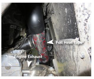
Apply foil heat tape around the snorkel where it comes in close proximity to the engine exhaust.
