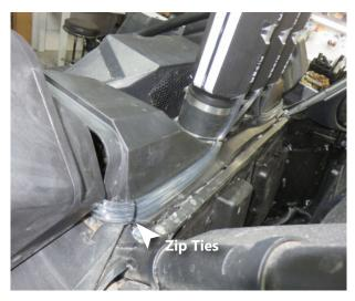
Secure the vent lines to the engine cover by drilling small holes in the cover and using zip
