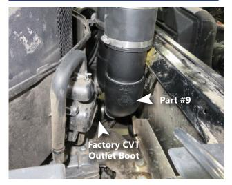
Beginning at the lower factory rubber boot on the belt housing, replace the factory hose clamp with a heavy duty hose clamp supplied in your kit.
