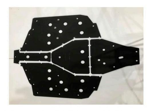
A. Remove the battery from the vehicle if it is not a sealed-cell battery. To ease installation, gently tip vehicle onto its side and support securely. Remove the OEM skid pan. Discard. Also, the metal tab where the front center of the OEM skid plate was attached will need to be bent up inside the center of the of the vehicle. Using pliers, dead-blow hammer, etc., bend enough to install the Trail Armor skid plates. See Picture 1.
