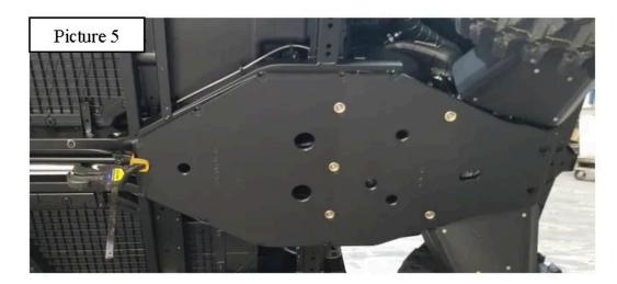
F. Locate Panel D of the skid set. Also, locate three OEM factory screws and three OEM bowl washers. Slide Panel D into position at the joints of Panels B and C. Insert one into the center hole to ease installation. Insert the other two after the panel is secure. See Picture 6. Loosely tighten. Repeat for the opposite side.
