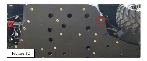
N. Locate one supplied #14 x 1" TEK self-drilling screw and one supplied bowl washer. Insert these into the remaining hole of the panel. See Picture 13. Repeat Steps K-N for the opposite slider.
