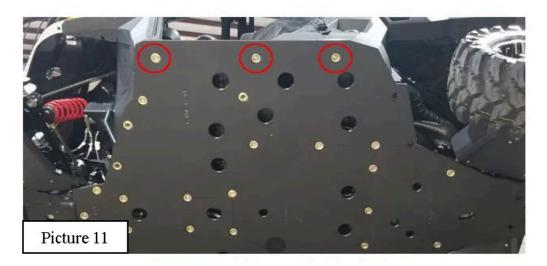
M. Locate one supplied ¼-20 x 1" serrated flange bolt, one supplied bowl washer, and one supplied ¼-20 t-nut. Insert these into the rear outside hole of the panel. The t-nut can be accessed from the rear of the frame rail. See Picture 12.
