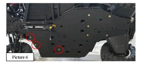
G. Locate Panel A from the skid set. Also, locate one supplied ½-20 x 1" serrated flange bolt, one supplied bowl washer, and one ½-20 t-nut. Remove the bar clamp and lay aside. Slide Panel A into position and insert the bolt and washer through the front hole of Panel A. Secure with the t-nut. The t-nut will need to be accessed from inside the frame rails. See Pictures 7A and 7B.
