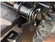
Step 3: Reinstall the Pivot Brackets with the bumper brackets into the tailgate assembly and tailgate using the provided 6mm Hex Bolt (note: leave all hardware very loose until the final step).
