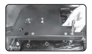
**STEP 6** With all four nyloc nuts started, ensure that the slider plate/tube assembly is square on the seat and positioned to the back of the seat, then tighten each through-tube nut securely (figure 6).
