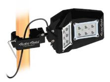
**Step 4** | Tighten bolts evenly to secure to cage. *Do not exceed 60 in/lb.* Route wire through clamp or between clamp & cage.
