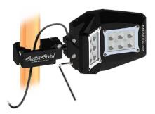
**Step 5** | Adjust mirror/light to preferred angle and then tighten adjustment screw to desired firmness. *Do not exceed 60 in/lb.*
