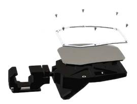
**Mirror Replacement** | To replace the convex mirror, first remove the six-M4 bolts, followed by the bezel, then carefully remove the convex mirror. Make sure to clean out any debris in the mirror cavity before replacing the mirror. To install new mirror, follow the previous steps in reverse. Tighten bolts incrementally in a diagonal pattern to reduce chance of glass breaking. Torque spec.: 70 in/lb.
