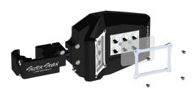
**Lens Replacement** | To replace either of the lenses, first remove the four-M4 bolts, followed by the bezel, then carefully remove the lens. Make sure to clean out any debris from the LED cavity and make sure that the O-ring is clean and clear of debris as well. To install new lens, follow the previous steps in reverse. Tighten bolts incrementally in a diagonal pattern to reduce chance of glass breaking. Torque spec.: 70 in/lb.
