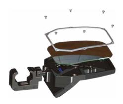
**Mirror Replacement** | To replace the convex mirror, first remove the six-M4 bolts, followed by the bezel, then carefully remove the convex mirror. Remove and discard additional piece of foam (if present). Make sure to clean out any debris in the mirror cavity before replacing the mirror. To install new mirror, follow the previous steps in reverse. Tighten bolts incrementally in a diagonal pattern to reduce chance of glass breaking. Torque spec.: 70 in-lbs. Note: Do not overtighten.
