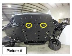
J. Locate seven supplied 14 x 1" TEK self-drilling screws and bowl washers. Insert these into the seven center holes of Panel D. See Picture 9.
