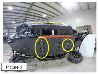
G. Working from front to rear, insert two supplied 14 x 1" self-drilling screws and bowl washers at the center of Panel A and three at the lap joint of Panels A and B. Next, insert five supplied 14 x 1" self-drilling screws and bowl washers at the lap joint of Panels B and C. See Picture 6. Leave the front two outside holes open. These will be installed in a later step.
