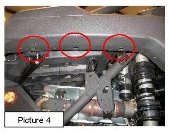
B. Prior to installation of the rear extensions, remove one OEM screw from the outside of the rear taillight housing. See Picture 3. Next, locate three supplied 1/4-20 U-nuts. Insert one into each of the three slots at the top of the fender well. See Picture 4.
