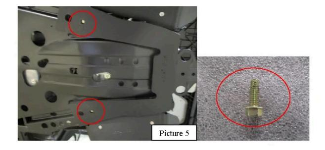
F. Locate Panel C of the skid set. Also, locate two supplied ½-20 x 1-1/2" thread cutting screws and two supplied bowl washers. Holding Panel C into position, insert these into the two center holes of the panel, through the front(larger) holes of the spacer into the u-nuts (highlighted in RED). Also, locate three supplied M6-1.0 X 30 mm. bolts and three supplied bowl washers. Insert these into the lap joint hole at the front of Panel C (highlighted in YELLOW). Loosely tighten. See Picture 6.
