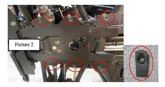
B. Locate six supplied 1/4-20 u-nuts from the supplied bolt pack. Insert these into the OEM holes between the front a-arms. See Picture 2.
