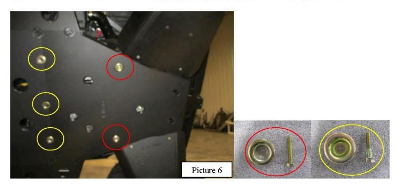
G. Locate Panel B of the skid set. Slide Panel B underneath the lap joint of Panel A. Next, slide Panel B towards the rear of the vehicle and under the M6-1.0 x 30 mm. bolts previously installed. We used a small bar clamp to temporarily hold Panel A and Panel B's lap joint together. If possible, use a small ratchet strap to tighten lap joints and ensure all panels are aligned properly. See Picture 7.
