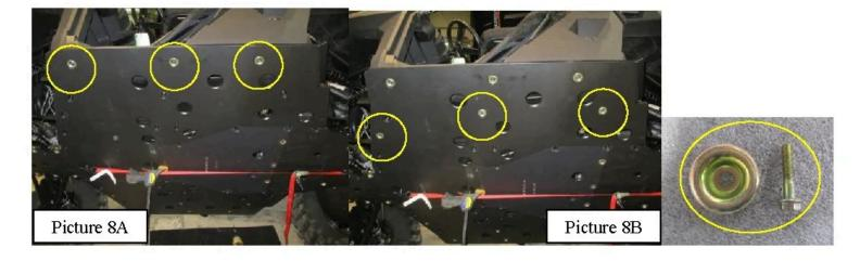
H. Locate Panel D of the skid set. Also, locate three supplied M6-1.0 X 30 mm. bolts and three supplied bowl washers. Slide Panel D's lap joint behind the lap joints of Panels A, B, and C. Insert these into the three outer holes of Panel D. Loosely tighten. See Picture 8A.
