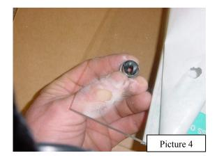
B. Insert supplied rubber grommets into the pre-drilled holes. See picture 4. Properly installed, the grommets' shoulder edges are uniform on both sides of the window. See picture 5.
