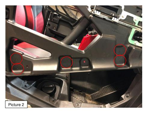
B. Locate the five drill points on the outside of the door panel. Using a ¼" drill bit, drill the five holes completely through the door panel. Make sure the door is open to keep from drilling into the seat! See Picture 2.
