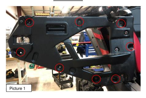
A. Remove door cover from the door frame by removing eight OEM screws as shown in Picture 1. Retain as they will be reused.
