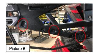
F. Locate five supplied ¼-20 x 1" Torx Truss screws and five ¼-20 nylock nuts. Slide the tabs of the extension up into the slots. From the inside of the door, insert one 1" screw through the door panel, through the extension, and secure with the ¼-20 nylock nuts. See Pictures 6 and 7.
