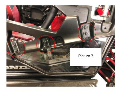
G. Replace the door cover and tighten securely but DO NOT OVERTIGHTEN! See completed install picture below.
